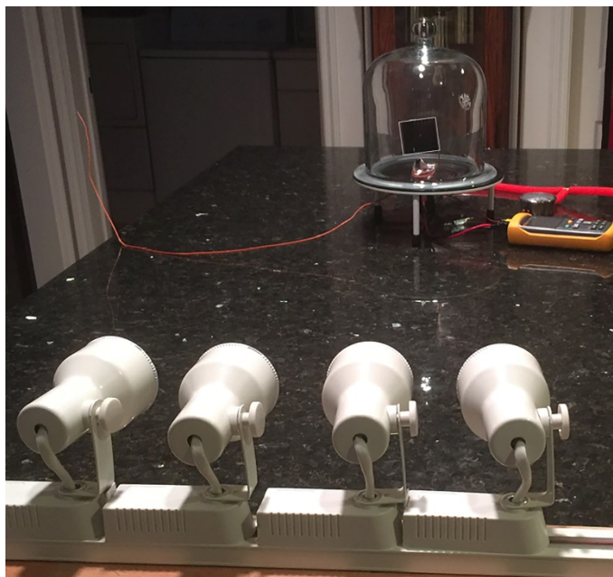
Figure S2. Four picture lights shining in a 2-inch square black metal plate inside of a vacuum jar.
